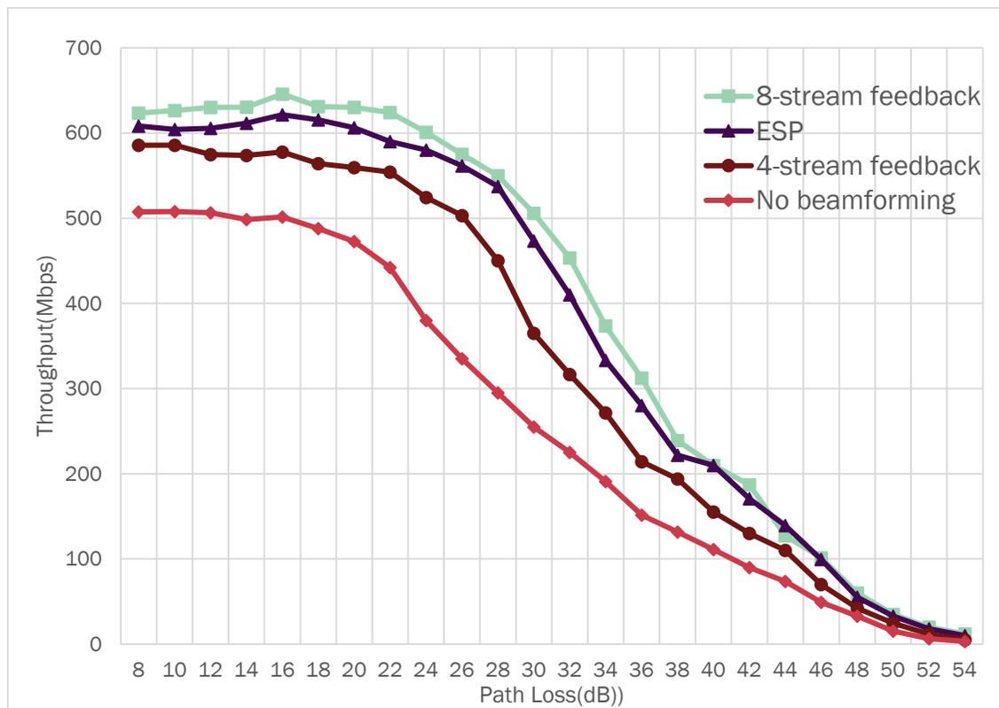
Figure 5: Comparison of Beamforming results for different types of channel feedback
