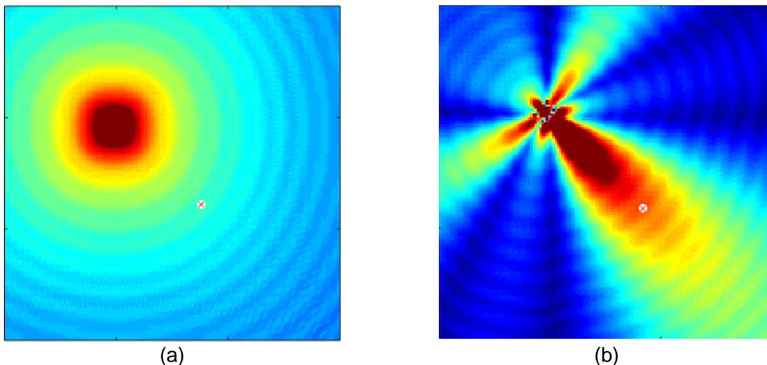
*Figure 1: two-dimensional illustration of Beamforming. Precoding directs the signal towards the intended receiver.*
