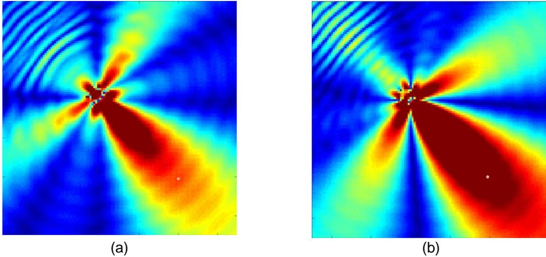
Figure 3: Illustration of BF gain with four antennas vs. eight antennas
