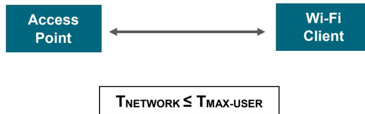
In these legacy Wi-Fi networks, consider two scenarios for doing speed test. In the first scenario, multiple devices are connected and are all simultaneously trying to do the speed test and in the second scenario, only a single device, the one with maximum throughput is connected and performing the speed test. The total aggregated throughput in first scenario will be definitely lower than the second one. This is due to two reasons,
