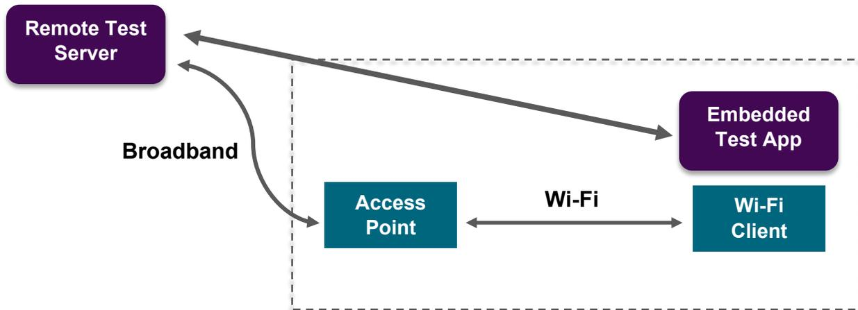
To properly isolate the Wi-Fi performance from the broadband speed, it is necessary to use a local test server attached to the access point, as illustrated below. Using traffic generation tools such as iPerf or Chariot to allow for accurate testing of Wi-Fi only traffic.
