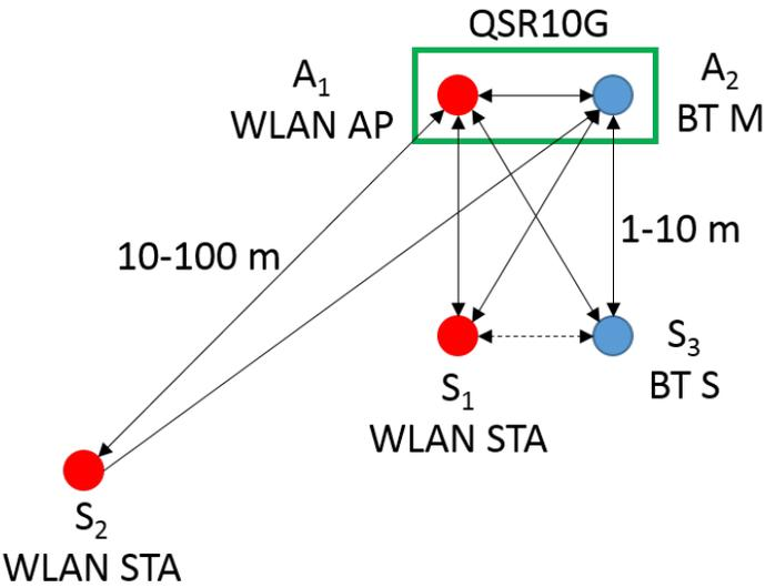
Figure 1. Example network with WLAN and BT clients connected to a QSR10G AP.
