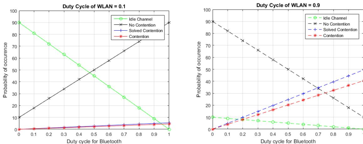
Figure 5. Probability of events with varying duty cycles of Bluetooth with 0.1 and 0.9 duty cycle of WLAN
