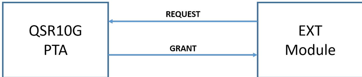
Figure 2. Quantenna's 4-wire interface between the QSR10G PTA and an external module.
